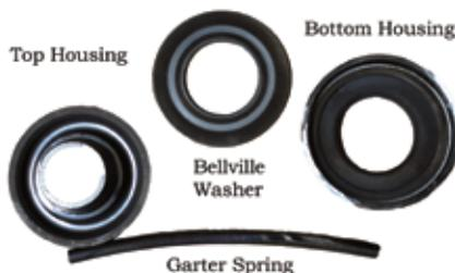
The rotator shown is a garter spring type found in most Continental engines. Most uneven heat signatures occur when the rotator stops working. When the valve stops rotating, the wear is concentrated in one spot on the edge of the valve. This leads to reduced heat transfer into the cylinder head and a subsequent hot spot.
