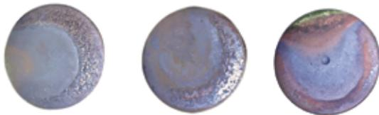
Late stage valves typically have U shaped or bell curve shaped deposits. The hot spot is in the center of the U or bell curve. Valve edges sometimes turn green at the hot spot. Late stage valves should be removed from service.
