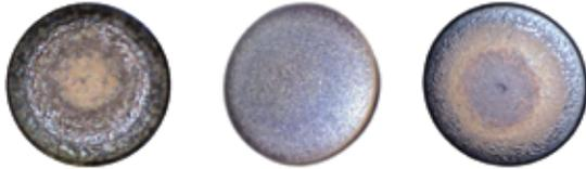
Normal heat signatures have a bulls eye pattern. Deposits can be thick or thin. Lean operation can make deposits hard to see. Rich operation will make thicker deposits. Color can vary from black, to grey or red.
