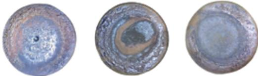
Early stage uneven heat signatures still have rings. The outer ring develops a gap at the hot spot. The center of the bullseye becomes elongated in the direction of the hot spot. Valves in this stage can typically be lapped in place to restore valve seating. Heat signature takes approx 30hrs to return to normal after valve is lapped.
