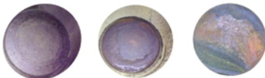
These valves had known operation in excess of redline CHT. High CHT typically results in two hot spots 180 degrees apart. Left and center photos are the same valve taken 47hrs apart. The uneven heat signature and head crack were not present right after the CHT event. Damage was not immediately apparent!
